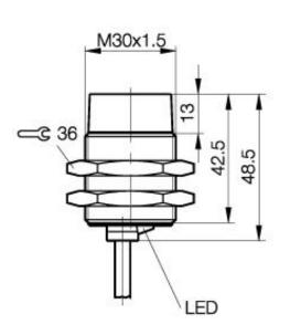
Inductive Sensors BES 516-3029-E4-Y-03 M30x1.5 x 48.5 normally-closed Sn=15mm unshielded
